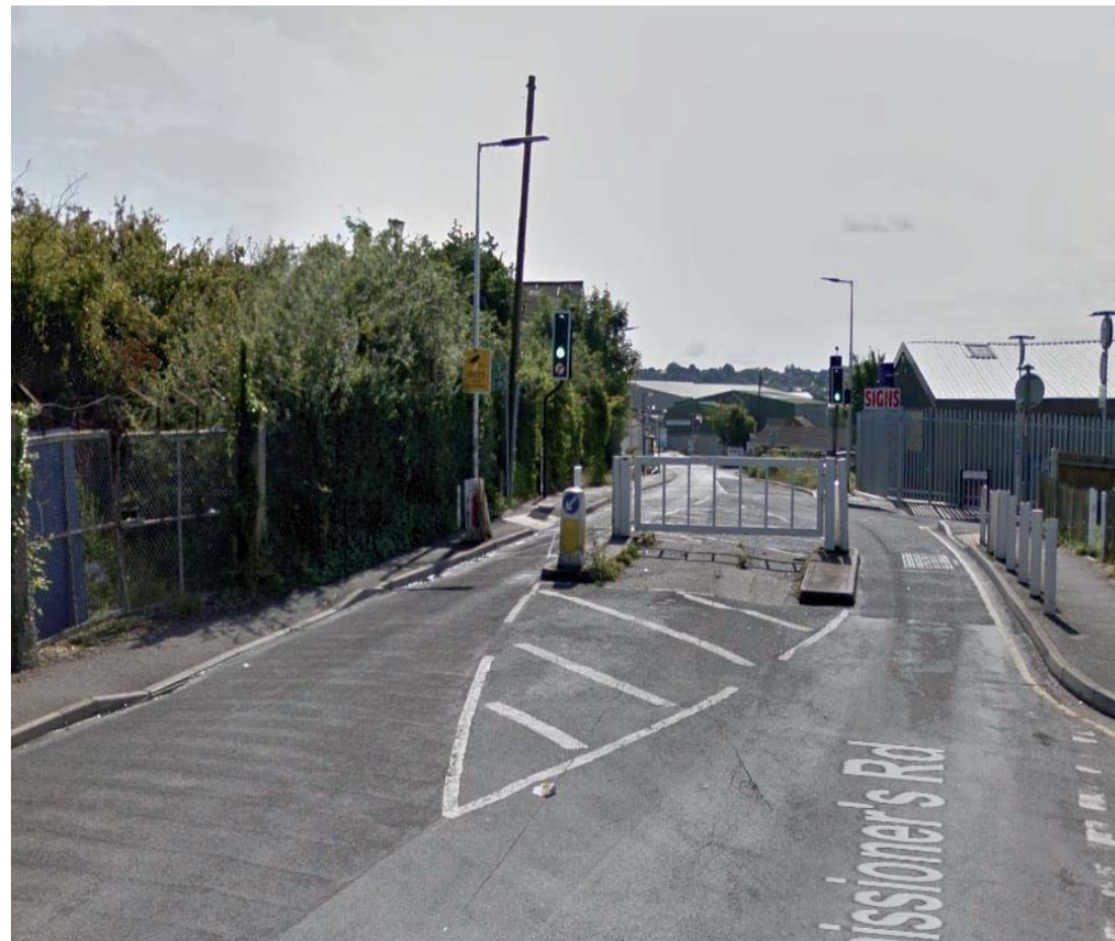
Above: Example of HGV prevention gates at Commissioner's Road, Strood Below: Passive design to prevent HGV access in an urban environment
